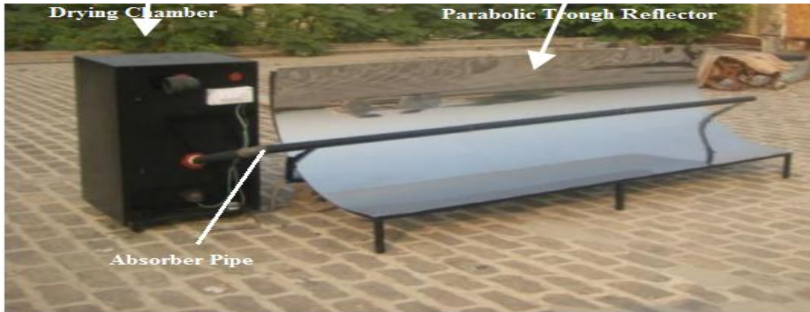
Fig 2. Isometric view of Parabolic Trough Solar Concentrator
